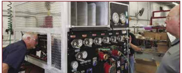
The compartment body being prepped for mounting to the chassis.
