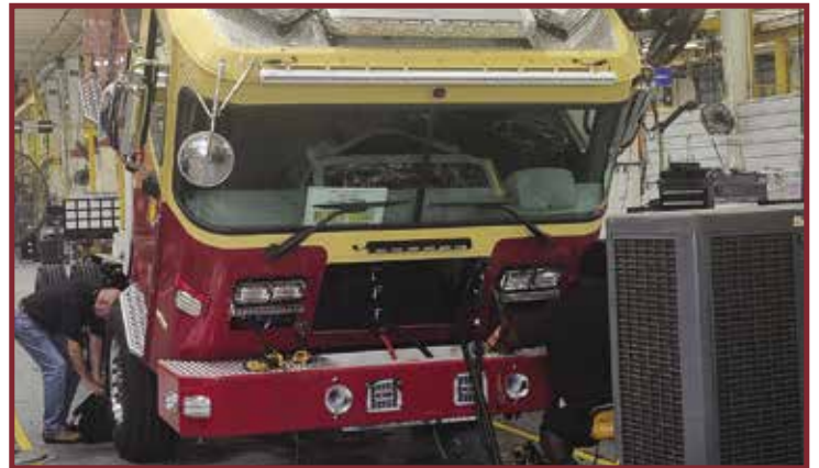
The cab being mounted to the chassis.
